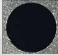
The CoroDrill® solution improved hole quality without delamination and splintering.
